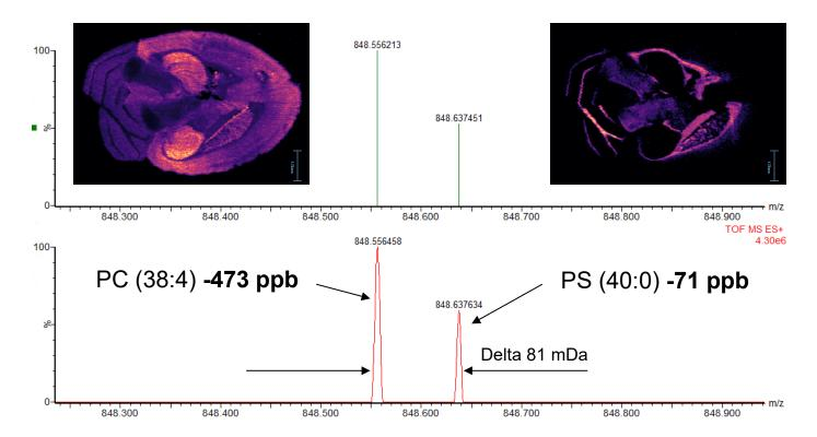
Figure 4: High mass resolving power allows interference-free biolocalization of two lipids that differ by only 81 mDa.  $PC(38:4) + K^+$ , expected mass: 848.556614, observed mass: 848.556213, mass error: -0.401 mDa, -473 ppb and  $PS(40:0) + H^+$ , expected mass: 848.637511, observed mass: 848.637451, mass error: -0.06 mDa, -71 ppb.
