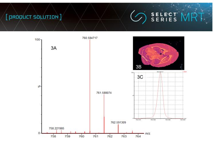
Figure 3A: DESI MS imaging spectra identified as PC (34:1), 3B: biolocalization of PC (34:1) and 3C: MS resolution, observed half height 0.003784 corresponding to >200,000 FWHM.
