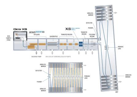
Figure 1: SELECT SERIES MRT instrument schematic.
