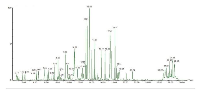
Figure 2. BPI chromatogram of tryptic digest of ENBREL (etanercept) analyzed via RPLC/HDMS<sup>E</sup> (single pass IMS).
