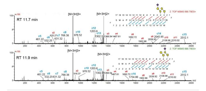
Figure 3. ECD MS spectra for LC-HDMS/MS peaks at RT 11.7 and 11.9 min (m/z 890.7, 3+). Selected m/z for T19 tryptic peptide (SMAPGAVHLPQPVSTR) with 2 HexNAc + 2 Hex + 1NeuAc. ECD fragmentation confirms locations and identities of two Core 1 O-glycans at positions 14 and 15.
