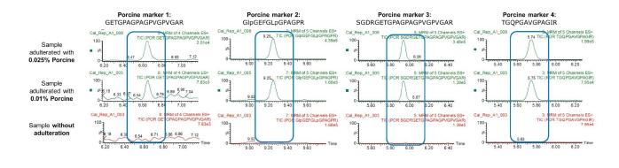
Figure 5. Comparison of MRM chromatograms for the four porcine markers in halal-labeled candy with and without the addition of the porcine gelatin standard.
