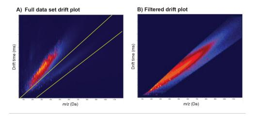
Figure 5. Top: Plots of drift time versus mass to charge (m/z) for the A) full data set for the effluent wastewater sample and B) filtered (area depicted in frame A within the yellow lines) for potential PFAS compounds. Bottom: C) Comparison of the base peak intensity chromatogram for the wastewater effluent sample before (top) and after (bottom) drift time and m/z filter was applied.
