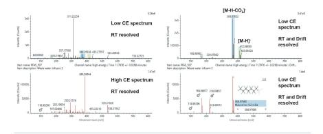
Figure 3. Low and high CE spectra for PFOA in the wastewater influent sample. Left are the spectra with alignment by retention time only and Right are the cleaner spectra having undergone retention time and drift time alignment. Fragment ions in the high CE spectrum can be associated with PFOA and the isotopically labeled standard.
