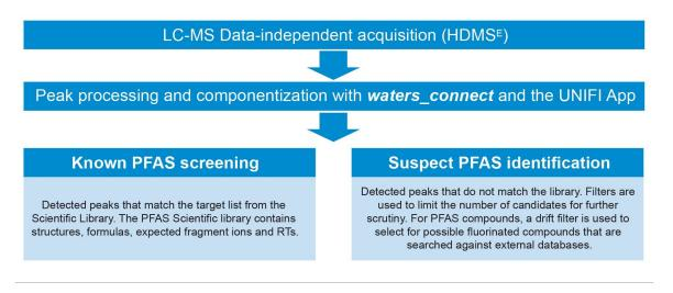
Figure 1. Schematic of the methodology used for PFAS identification in environmental samples with LC-IMS-MS.
