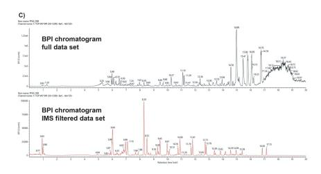
Figure 5. Top: Plots of drift time versus mass to charge (m/z) for the A) full data set for the effluent wastewater sample and B) filtered (area depicted in frame A within the yellow lines) for potential PFAS compounds. Bottom: C) Comparison of the base peak intensity chromatogram for the wastewater effluent sample before (top) and after (bottom) drift time and m/z filter was applied.
