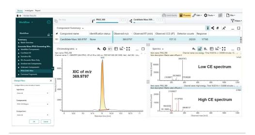
Figure 6. An example of a candidate compound (m/z 369.979, RT 10.01 min) revealed in the wastewater effluent sample using the drift time vs m/z filter. The low and high CE spectra are aligned by RT and drift time for candidates and are used for structural elucidation with tools in UNIFI.
