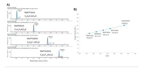
Figure 9. A) XICs for a series of related compounds (MePrSAA, MeFBSAA, MePeSAA, and MeFHxSAA) that were detected in the same wastewater effluent sample. B) Plot of calculated CCS versus m/z for the compounds and N-MeFOSAA which has a CCS value based on an authentic standard.
