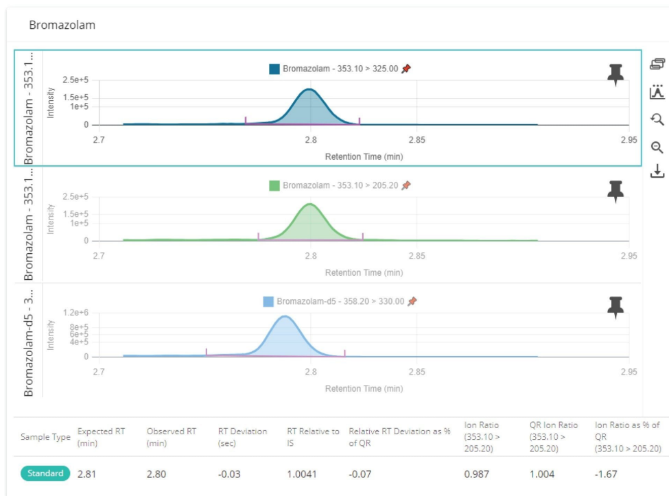
Figure 3. QUAN review peak integration review window for Bromazolam at 5 ng/mL. The quantifier, qualifier and internal standard transitions are displayed, above the acceptance criteria for retention time and ion ratio.
