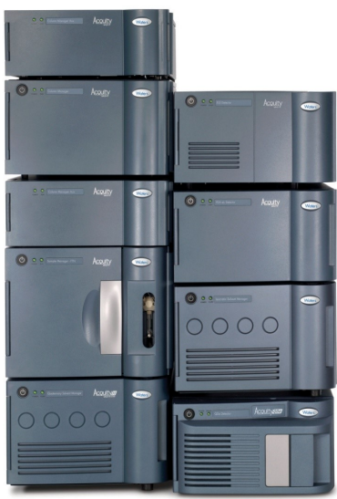
Figure 1. ACQUITY UPLC H-Class system with triple detection including ACQUITY PDA, ELSD and QDa detectors. The triple detection system includes an isocratic solvent manager (ISM) which provides make-up solvent to the QDa detector and houses the splitter required for the ELSD and the QDa. After the PDA detector, the flow is split to the ELSD detector and QDa. The composition and flow rate of the make-up solvent impact the split ratio to the ELSD and the QDa.
