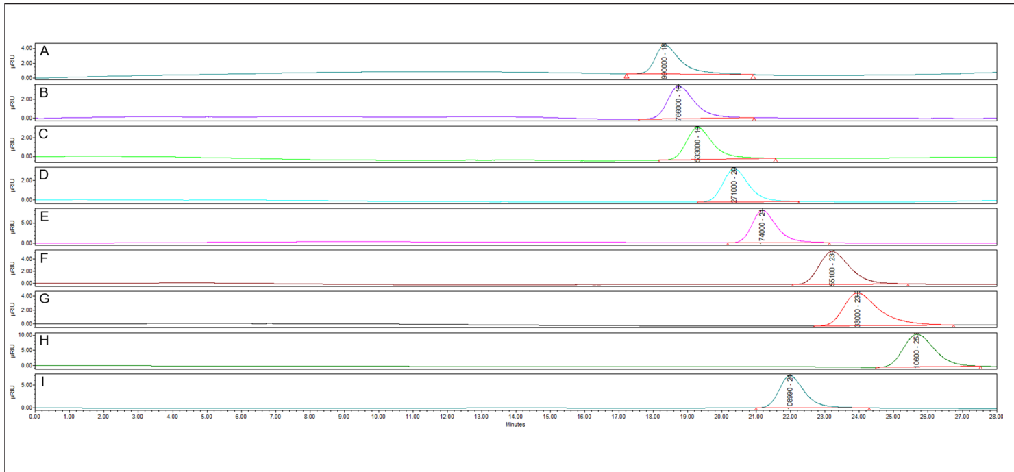
Figure 1. GPC analysis of narrow PMMA standards (A) Mp 990000 Da, (B) Mp 766000 Da, (C) Mp 533000, (D) Mp 271000 Da, (E) Mp 174000 Da, (F) Mp 55100 Da, (G) Mp 33000 Da, (H) Mp 10600 Da and (I) the broad PMMA sample (10800 DA) obtained on the Arc HPLC System equipped with strong solvent kit.
