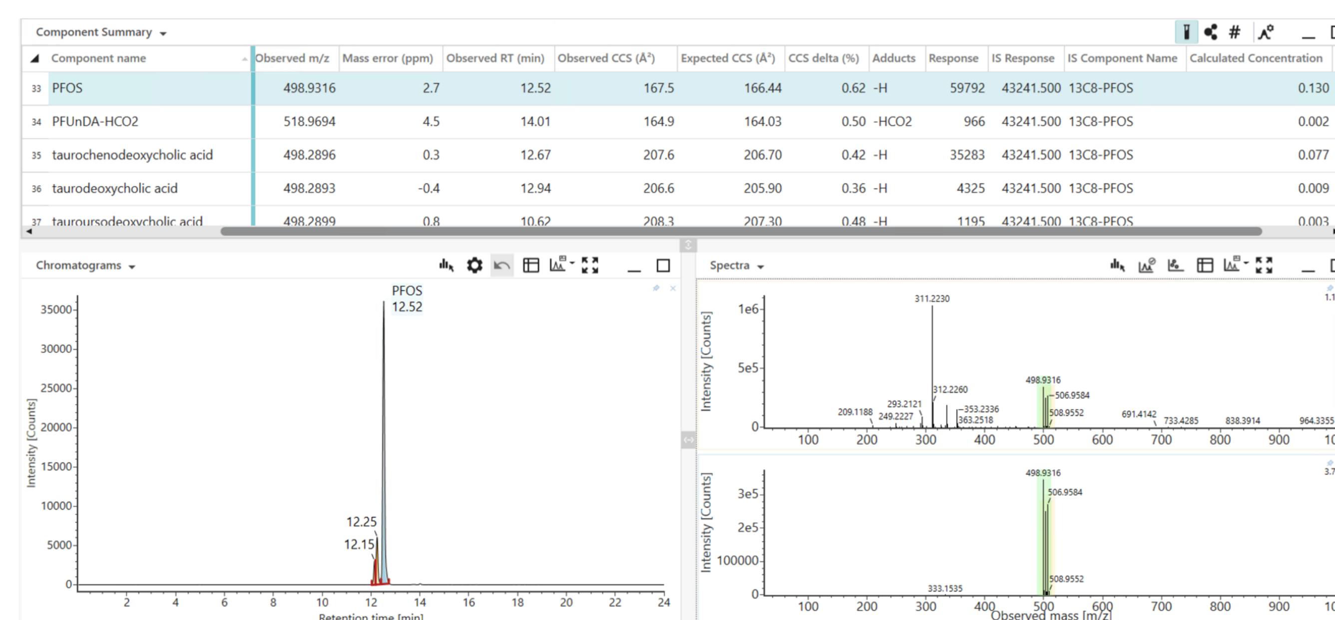
Figure 2. Component summary showing the calculated PFOS concentration (0.13 ng/mL) in firefighter sample F12 (Δ CCS = 0.62%). The mass spectra (right) include an ion mobility-resolved region (lower pane), enabling separation of PFOS ions from co-eluting matrix background signals (upper pane), and discrimination of native PFOS (C 8 HF 17 O 3 S), the (C 4 [ 13 C] 4 HF 17 O 3 S) injection internal standard, and the ([ 13 C] 8 HF 17 O 3 S) extraction internal standard.
