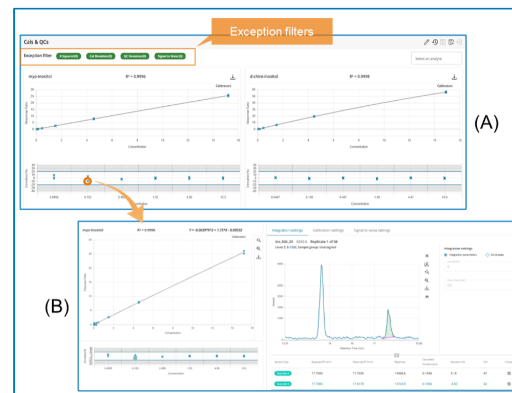
Figure 4. Screenshots of the Peak Integration Overview (A) and the individual injection peak integration review (B), accessible by clicking on the chromatogram image on the Overview page (indicated by the arrow). Exception filters are shown on the Peak Integration Overview page.
