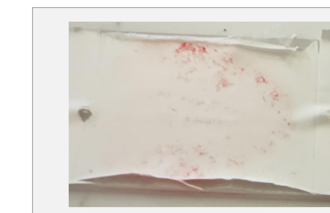
Figure 5. photograph of the nitrocellulose membrane after one DESI acquisition, with damage to the edges of the substrate shown.
