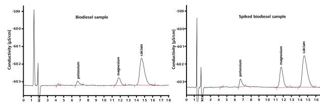
Sample Prep.: Extraction with 2 mol/L HNO<sub>3</sub> (15 min)
