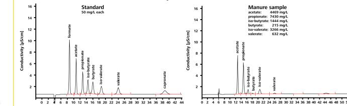
Sample Prep.: 1:100 dilution with ultrapure water injection after dialysis (10 min)
