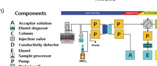
The continuous flow-through dialysis cell can be directly connected to the injection valve of the IC instrument.
