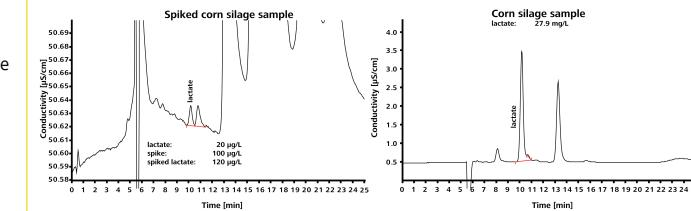
In contrast to the manure sample, the silage samples were diluted 1:50 and subsequently filtrated. The other experimental conditions were kept constant.
