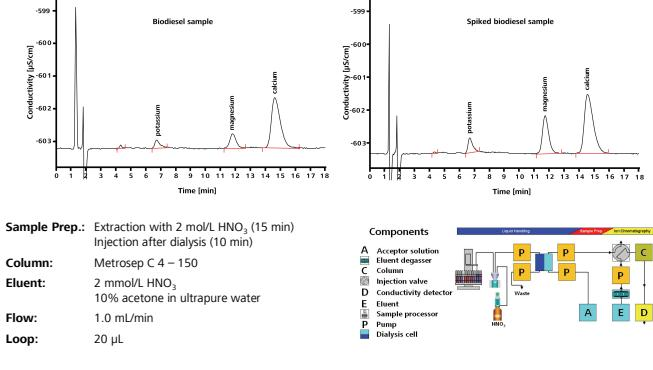
The continuous flow-through dialysis cell can be directly connected to the injection valve of the IC instrument.
