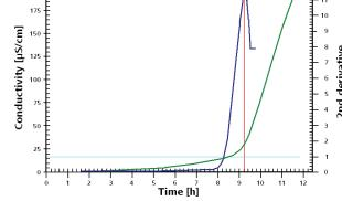
At 110 °C the investigated biodiesel sample has an induction time of 9.25 h. It thus complies with the minimal requirements of EN 14112 in EN 14214 (6 h) and ASTM 6751 (3 h).
