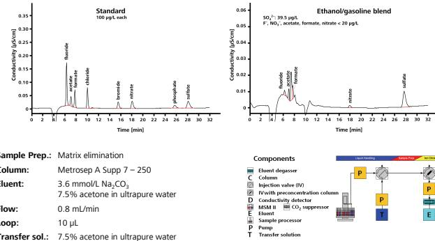
While the organic ethanol/gasoline blend is washed away, the analyte ions are retained on the preconcentration column.
