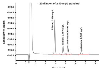
After a 1:20 dilution of the 10 mg/L calibration standard, the sample was automatically injected.
