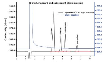
Carryover in the mixing vessel was evaluated by injection of a blank (ultrapure water) immediately after injection of a 10 mg/L standard.
