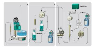
The sample is drawn through the injection valve (1) into the buffer volume (2). After switching the valve to the fill position, the exact volume is fed onto the preconcentration column (3). From there, the ions are eluted to the separation column (4).
