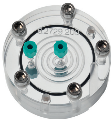
Figure 78: Top view of the low-volume dialysis cell, the simple but highly efficient purification system for complex samples.
