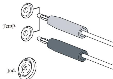
Figure 23 Connecting a temperature sensor
