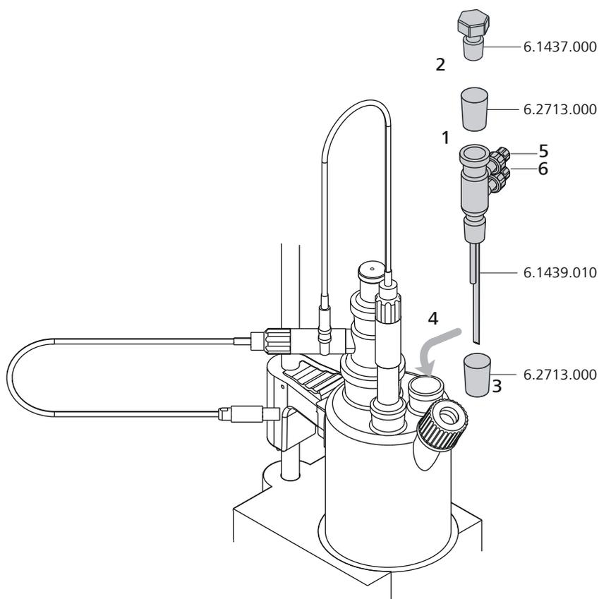
Figure 19 Mounting the addition and aspiration tube
