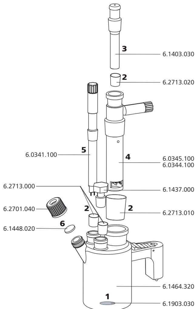
Figure 15 Equipping the coulometer cell
