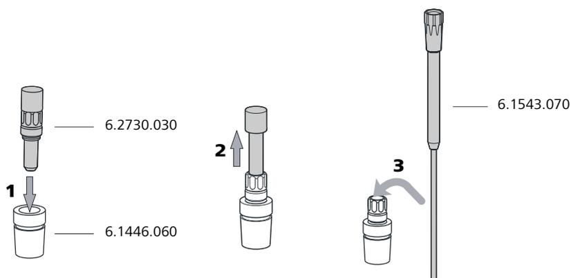
Insert the aspiration tip into the coulometer cell as follows:
