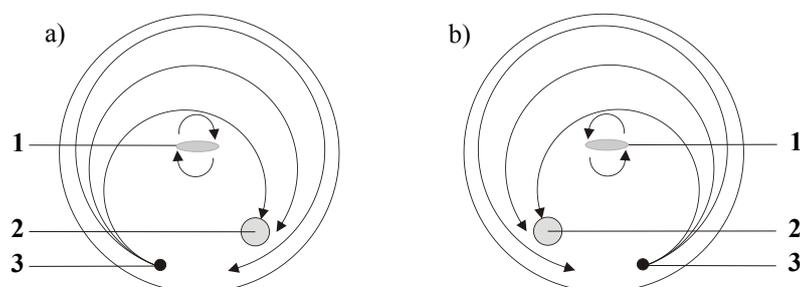
Figure 12 Schematic configuration of magnetic stirrer, indicator electrode and buret tip (Volumetry) / Generator electrode (Coulometry) during a titration. a) stirring direction clockwise, b) stirring direction counterclockwise.
