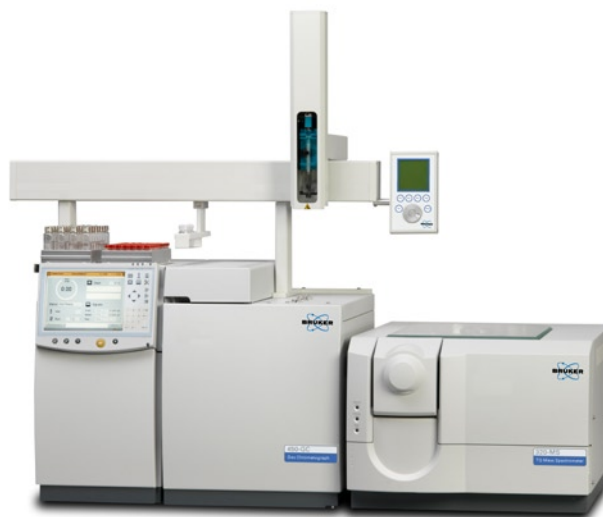
Figure 2: Bruker 300-MS triple quadrupole mass spectrometer with 450-GC gas chromatograph and CTC Combi PAL autosampler.
