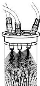
Illustration 18: Installation of rinsing nozzles
