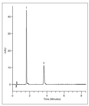
Figure 1: Chromatogram for 1. fenoprofen and 2. gemfibrozil separated on an Accucore RP-MS 2.6  $\mu$ m 100 x 2.1 mm column
