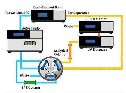
Figure 5. Flow schematic of on-line SPE.
