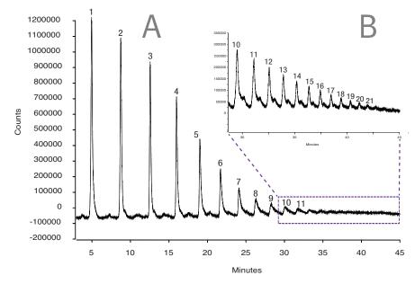
Figure 3: 2-AB dextran ladder separation. (A) 2 µL injection of sample, where 11 glycans were separated. (B) 5 µL injection of sample, zoomed-in to the later part of the gradient rise. A further 10 glycans were detected.
