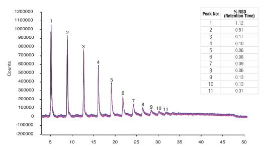
Figure 2: Overlay of triplicate runs of 2-AB labeled dextran ladder. Excellent reproducibility was found, further shown by the outstanding % RSD values (top right inset).
