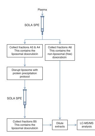
Figure 2: General scheme for the separate extraction of liposomal and non-liposomal (free) doxorubicin from plasma
