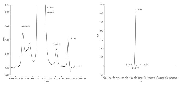
Figure 1B. Rituximab SEC separation, expanded view (left), full range chromatogram (right).
