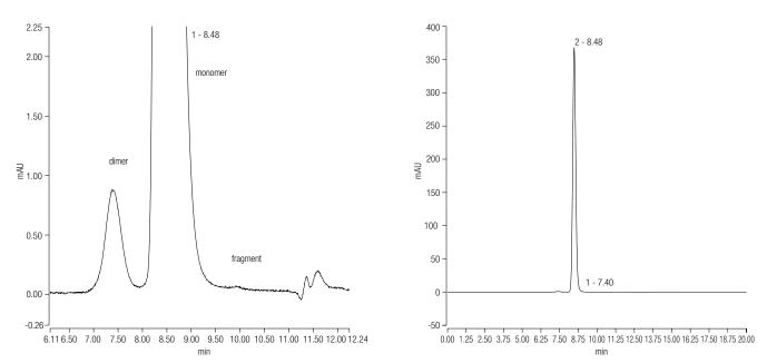
Figure 1A. Trastuzumab SEC separation, expanded view (left), full range chromatogram (right).
