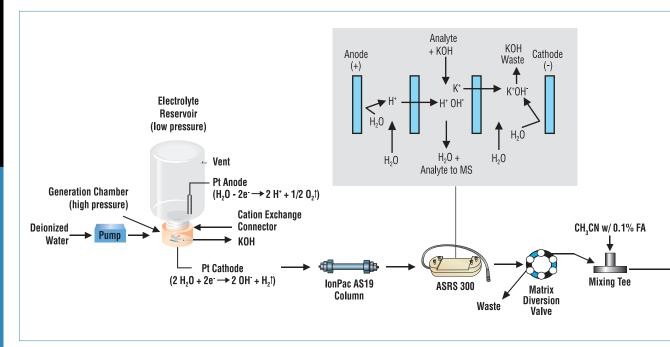
Figure 1: Flow schematic of the IC-MS/MS system
