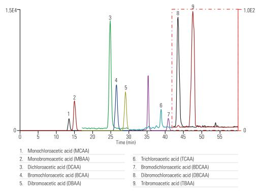
Figure 3: Separation and detection of the nine haloacetic acids using an ISC-3000 system with an lonPac AS24 column, coupled to a TSQ Quantum Access MS/MS system. Analyte levels were 2.5 ppb each in deionized water with an injection volume of 100  $\mu$ L.
