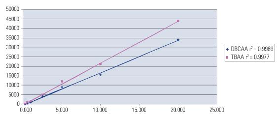
Figure 5: Overlay of calibration curves of dibromochloroacetic acid and tribromoacetic acid in water by IC-MS/MS
