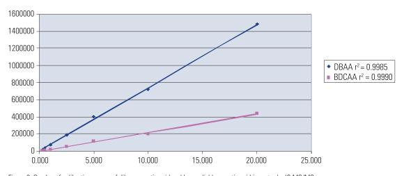
Figure 6: Overlay of calibration curves of dibromoacetic acid and bromodichloroacetic acid in water by IC-MS/MS
