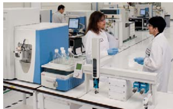
Figure 2: LC/MS analysis was performed using an Accela™ U-HPLC system coupled to an Exactive benchtop Orbitrap mass spectrometer
