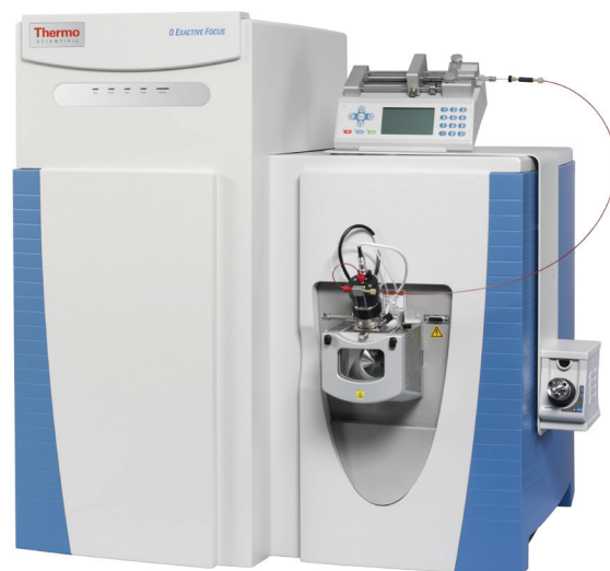
Figure 1. Q Exactive Focus benchtop Orbitrap mass spectrometer.
