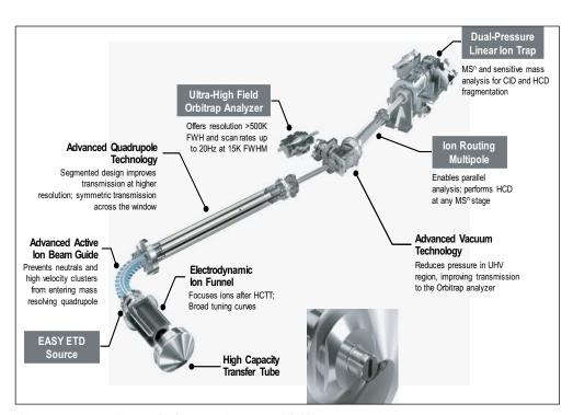
Figure 1. Instrument layout of Orbitrap Fusion Lumos Tribrid mass spectrometer.
