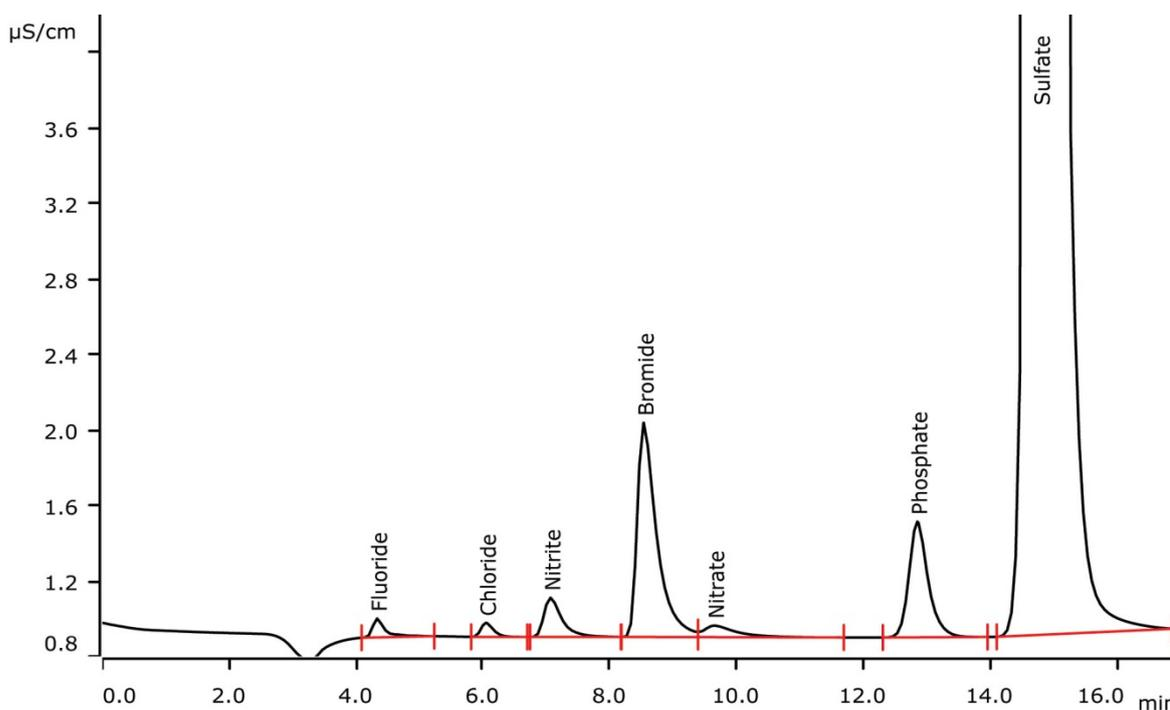
Determination of fluoride, chloride, bromide, and sulfate in a residual solvent applying combustion as sample preparation with subsequent anion chromatography with conductivity detection after sequential suppression. Analysis is crucial for waste classification in halogen-free and halogen-containing solvents.
