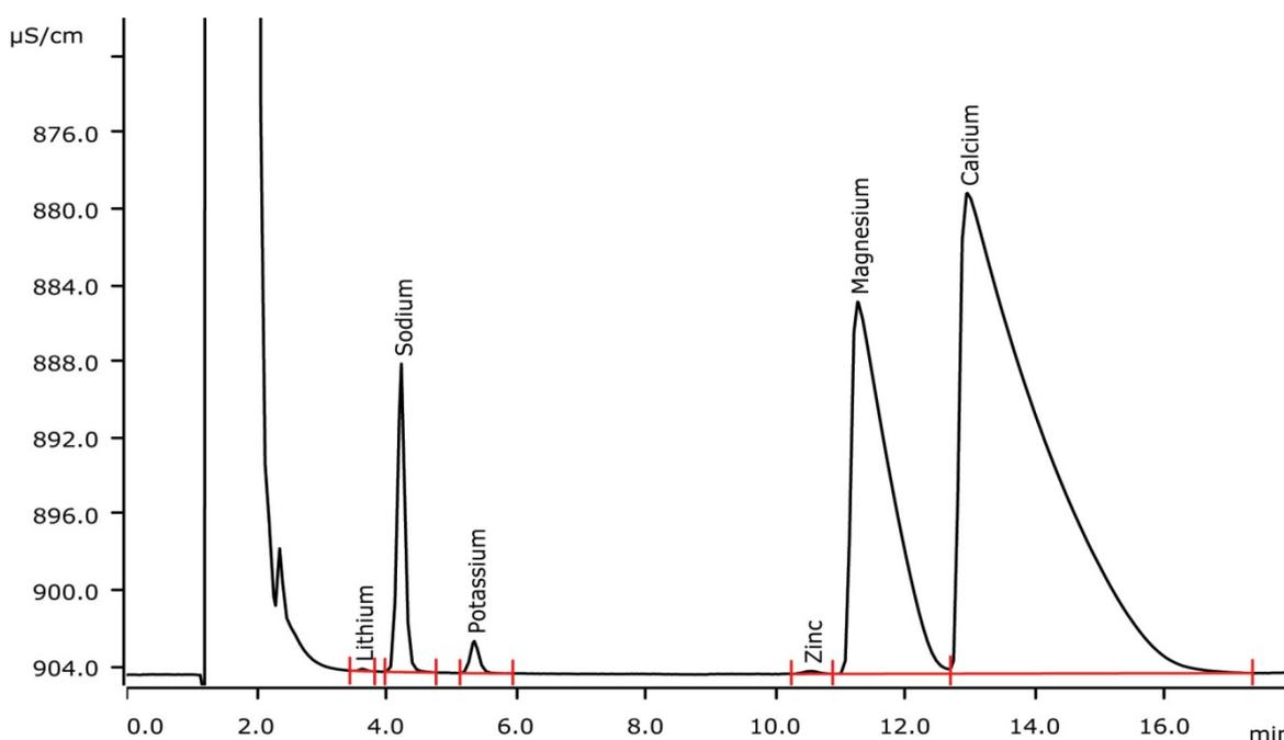
With Metrohm intelligent Pick-up Technique (MiPuT), the determination of cations in small sample volumes is straightforward. MiPuT allows to inject a very small aliquot of a very limited sample volume: only 10 µL out of 100 µL sample are required. Calibration is performed by injecting different volumes of a single mixed standard solution. For corresponding anion determination, see AN-S-302.
