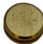
Figure 3 - one of the four test resistors. The number 100 refers to the approximated resistance, 100 \Omega .
