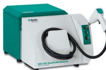
Fig. 3: The NIRS XDS SmartProbe Analyzer was used for raw material identification, such as for the identification of the final product.
