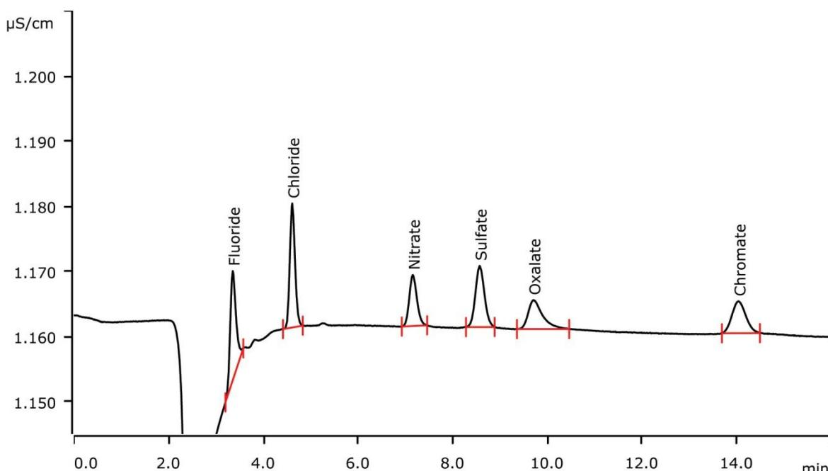
Water of the water-steam circuit of boiling water reactors (BWR) needs to be free of corrosive anions. Analyzing these trace anions allows the parallel determination of chromate, which is a potential corrosion product. Automated sample preparation includes variable Inline Preconcentration (MiPCT) and automatic calibration with a single multi-ion calibration standard.
