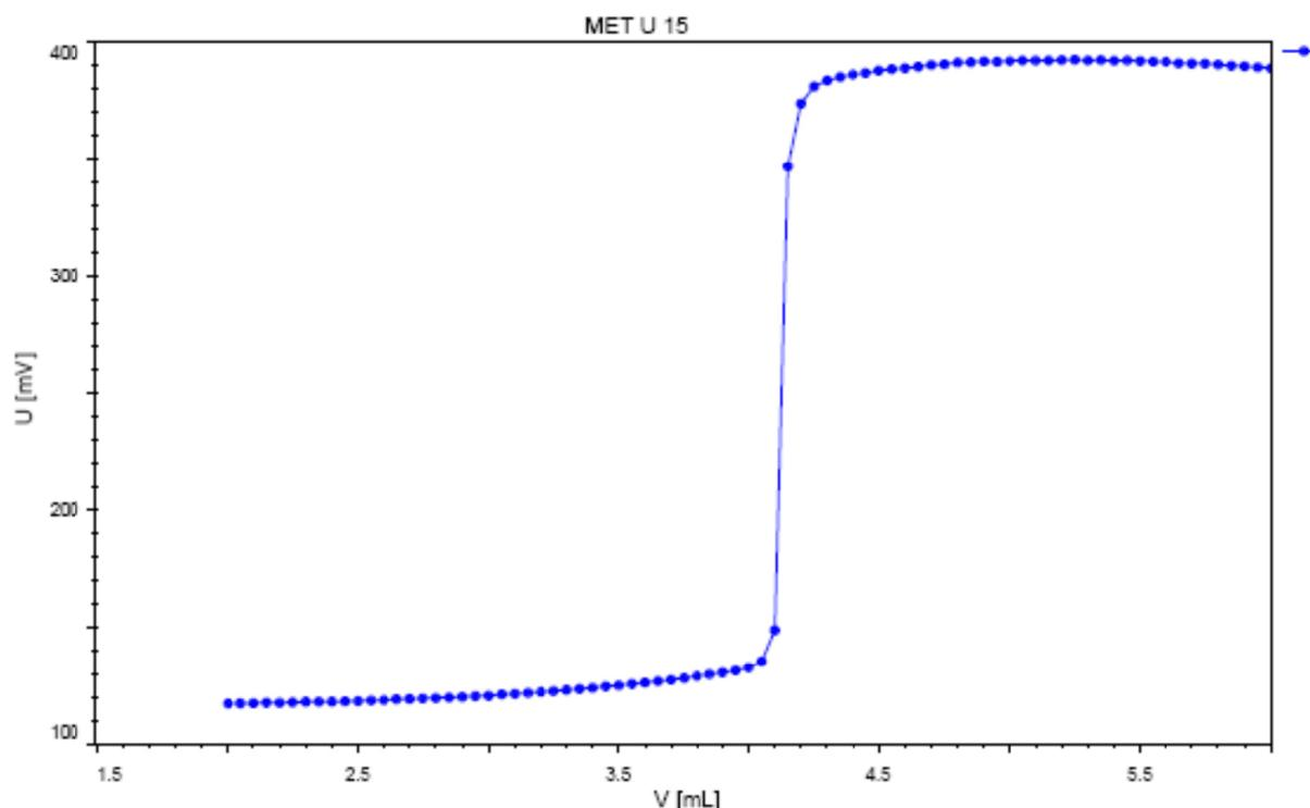
This Application Note describes the photometric determination of magnesium in cement by using the Optrode (610 nm). After digestion of a cement aliquot, magnesium is titrated with EDTA.
