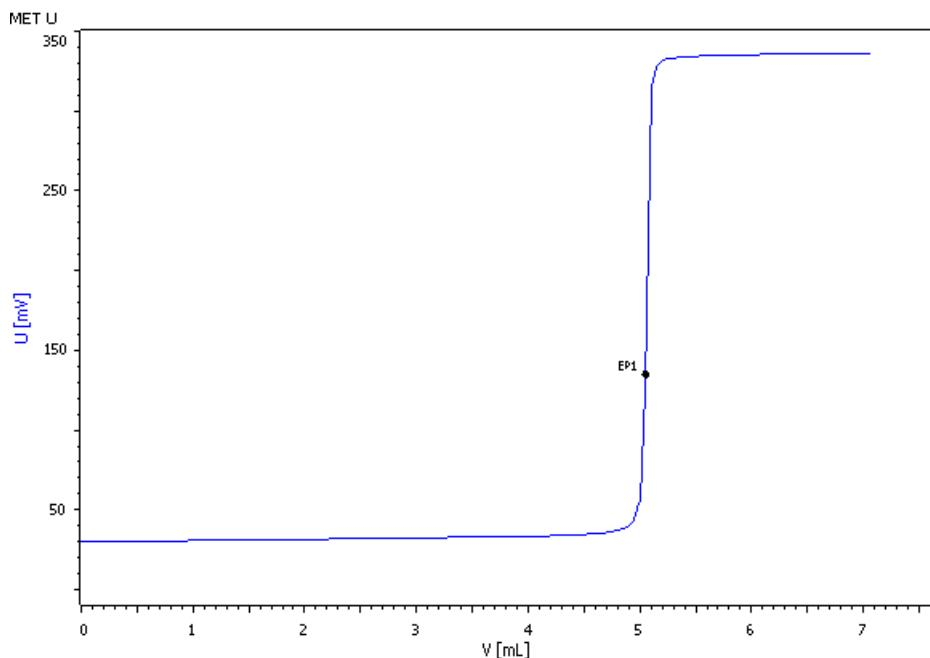
Barium can be determined in alkaline media by direct titration with EDTA. Phthalein purple is used as indicator; the equivalence point is determined with the Optrode at a wavelength of 574 nm.
