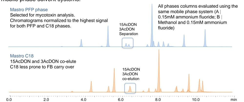
**Figure 3**. 18 Mycotoxins separated on a PFP phase compared to a C18 bonded material using ammonium fluoride as the mobile phase. PFP phases delivered near baseline resolution of 3-and 15 acetyldeoxynivalenol which is not possible on a C18 phase (C18 material can still be used due to preferential ionisation of 3AcDON in negative ion mode).
