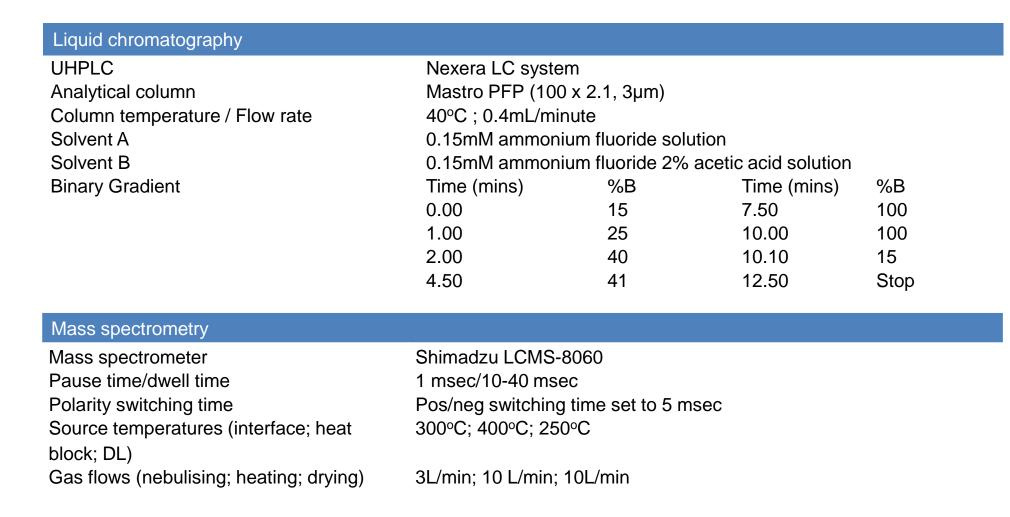
**Table 1**. LC and MS/MS acquisition parameters used to create the LC-MS/MS method.
