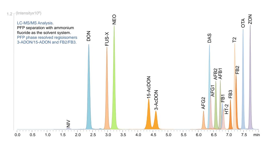
**Figure 1**. MRM chromatograms of 18 mycotoxins using a PFP bonded phase.
