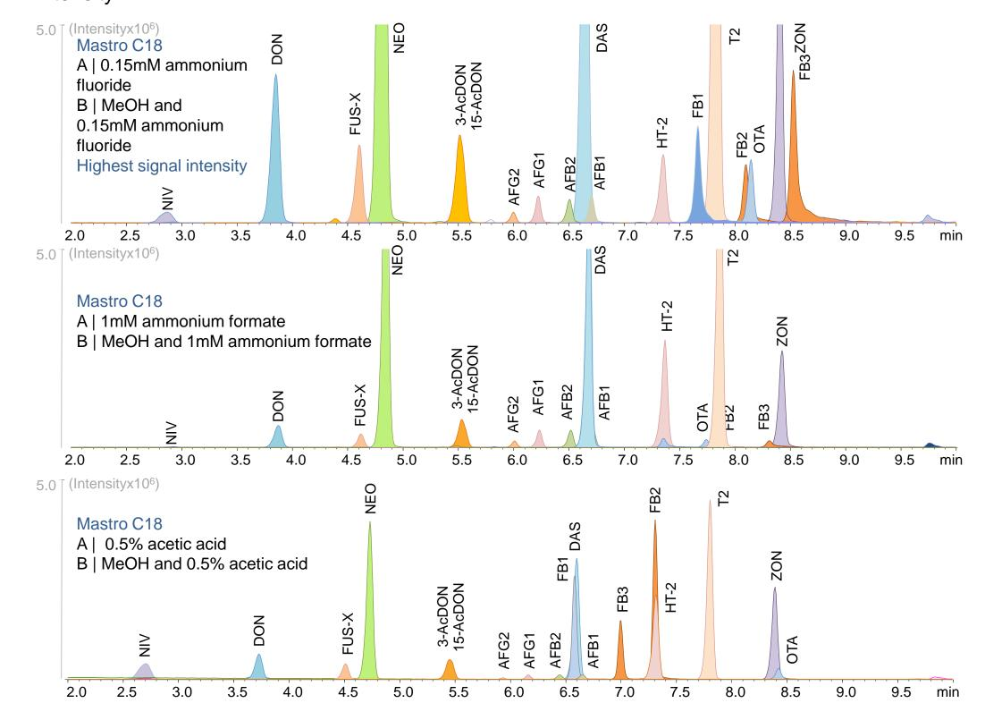
**Figure 2**. Ammonium fluoride markedly increases ion signal intensity compared to other solvent systems. All chromatograms are normalized to the same signal intensity. Ammonium fluoride delivered higher ion signal response for mycotoxins in positive ion mode compared to other mobile phase solvent systems.
