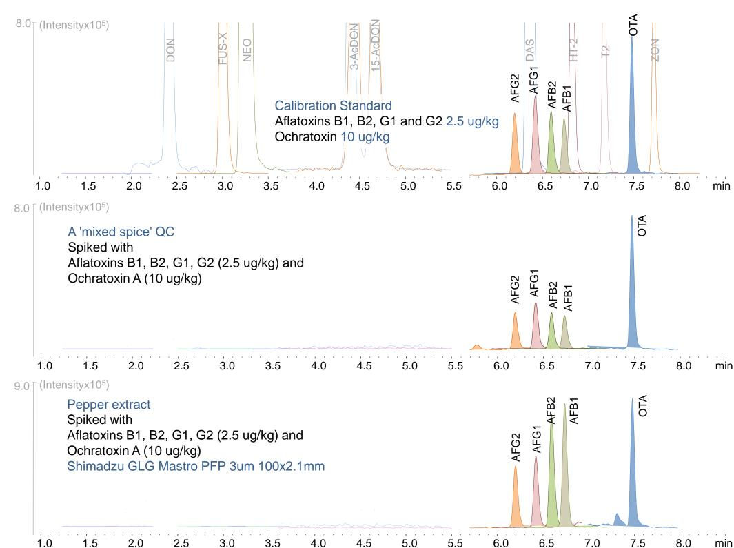
**Figure 4**. Analysis of a mixed spice extract and a pepper extract spiked with Aflatoxins B1, B2, G1, G2 (2.5 ug/kg) and Ochratoxin A (10 ug/kg) using ammonium fluoride solution in the mobile phase. Repeatedly injecting the extracts resulted in a %RSD typically below 10% (n=12) for Aflatoxins B1, B2, G1, G2 (2.5 ug/kg) and Ochratoxin A (10 ug/kg).
