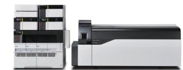
LCMS-8050 triple quadrupole mass spectrometer
