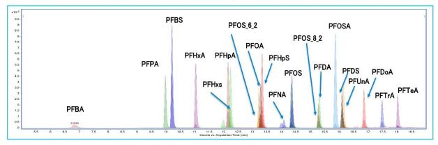
Figure 4. Standard of 19 PFCs with 100 ng/L for Large volume injection 400 uL
