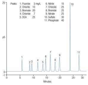
Figure2.Separationofcommonanions,DBPs,andDCAusingtheDionexIonPac AS27 column with a hydroxide gradient.
