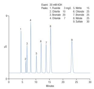
Figure 1. Dionex lonPac AS27 column QAR separation using an isocratic KOH eluent.
