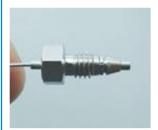
Once you are sure your fitting is complete, loosen the nut and inspect the ferrule for correct position on the tubing.
