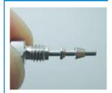
Carefully slide the ferrule components on after the nut. Finger-tighten the assembly while making sure the tubing is completely seated in the bottom of the end fitting.
