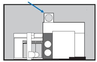
The connecting duct should provide unrestricted flow for the oven air and be as short and straight as possible.
