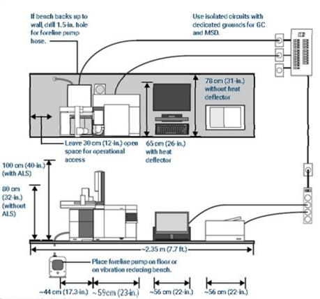
Typical GC/MS System - 8860 GC, 5977 MSD, with computer and
