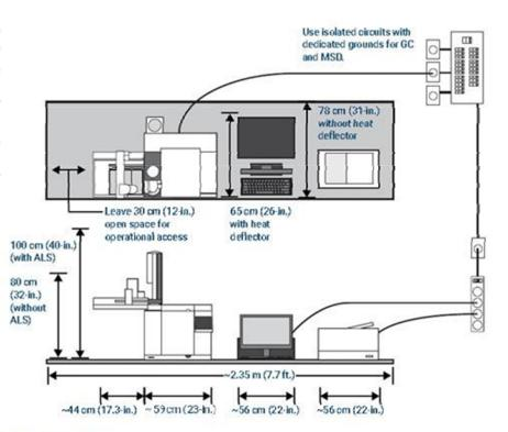
Typical GC System - 8860 GC with computer and printer.
