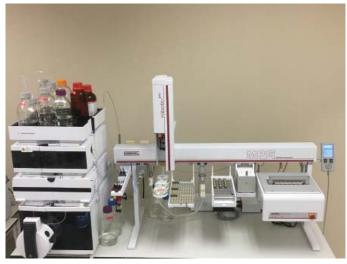
*Figure 1. MPS robotic*<sup>PRO</sup> *Multi-Purpose Sampler with the GERSTEL CF-200 centrifuge option.*
