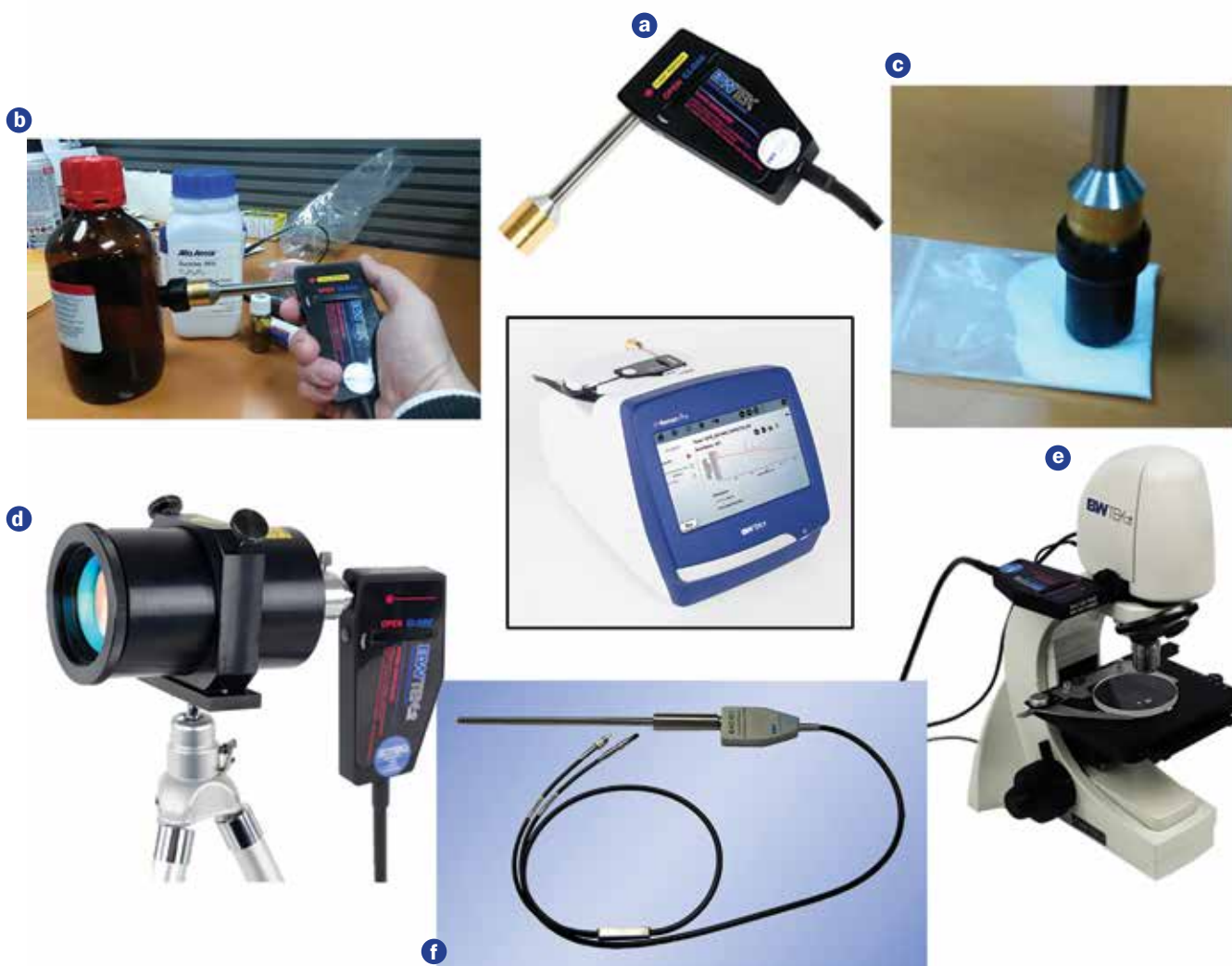
Figure 4. STRaman technology has the versatility to be used with a range of sample accessories to address different sampling needs. The standard STRaman fiber probe has a 4-mm diameter spot size (a). For measurement of liquids in glass bottles, the probe can be converted to the confocal configuration by adding the focus adaptor (b). Focusing on the sample deep inside the glass container maximizes the Raman signal while minimizing the fluorescence interference due to the glass. Adding a surface regulator on top of the focus adaptor (c) brings the focal point to the surface, making it easy to do everyday measurements of samples exposed or inside thin transparent packaging material. Replacing the STRaman probe shaft with a telescope lens allows for standoff Raman measurements (d). The same probe mounted on a microscope allows for Raman microscopy (e). Replacing the entire STRaman probe with an industrial grade probe (f) turns the instrument into a process analytical technology tool.
