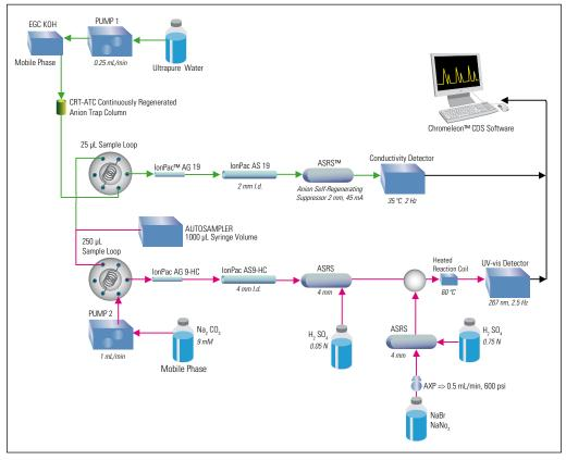
Figure 1. General representation of the chromatographic system.
