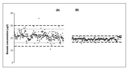
Figure 4. Control chart for bromate at a concentration of 20 µg/L. (A) Conductivity detection (chromatographic conditions 1); (B) Postcolumn reaction and UV-vis detection (chromatographic conditions 2).
