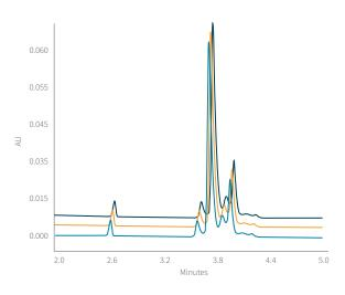
Trastuzumab charge heterogeneity profile separated utilizing the CZE Rapid Charge Variant Analysis Kit.
