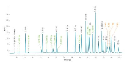
Separation of virus and plasmid DNA utilizing SCIEX dsDNA 1000 kit (Sample peaks are in green with DNA ladder peaks in black font.)
