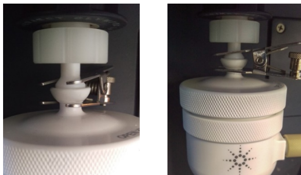
Figure 5. Installing the inert spray chamber onto the fully demountable ICP-OES inert torch. The procedure is the same on the semi-demountable ICP-OES inert torch.
