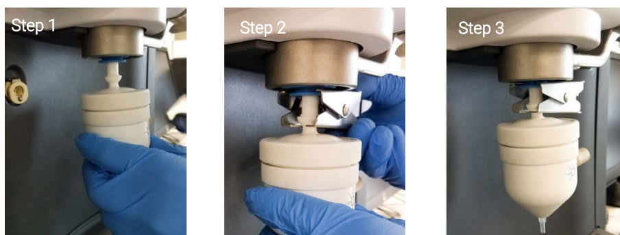
Figure 4. Installing the inert spray chamber onto the MP-AES inert torch.
