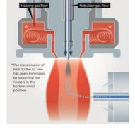
Figure 3. Heated ESI probe
