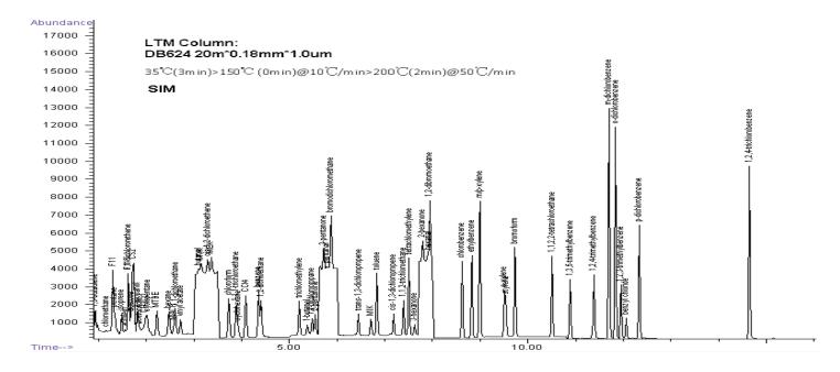
16 min for 60 VOCs MDL: 0.019~0.218 ppbv
