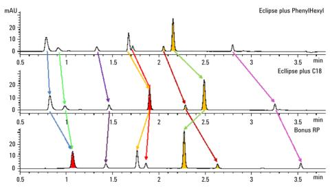
**Figure 3** Totally different chromatographic results by using the same sample but three different stationary phases
