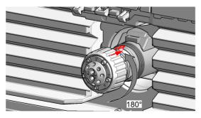
**2** When the outer pin is locked into the groove, manually screw the nut onto the valve head.
