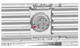
**4** Push the valve head until it snaps in and stays in the rear position.
