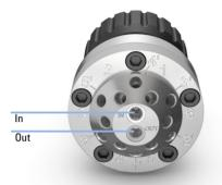
The *In* port is hydraulically connected to the column inlet ports 1-6 on the inner ring while the *Out* port connects to the column outlet ports  $1^-6^$  on the outer ring.
