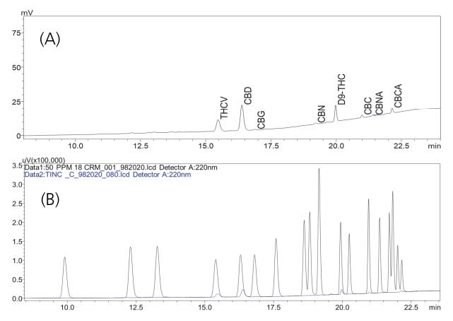
Figure 10: Tincture 2 profile (A); Tincture (blue trace) 1000x diluted vs. 50 ppm 18-Component Standard (black trace) (B). Results obtained at 5  $\mu$ L injection volume
