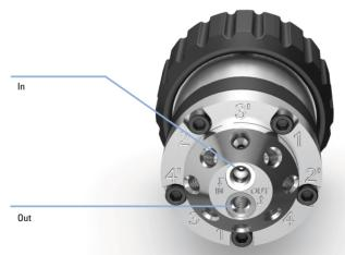
The *In* port is hydraulically connected to the column inlet ports 1-4 while the *Out* port connects to the column outlet ports 1`-4`.
