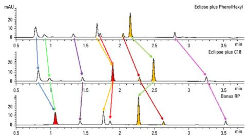
Figure 2 Totally different chromatographic results by using the same sample but three different stationary phases
