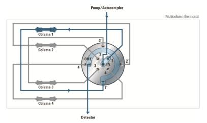
Figure 3 Hydraulic flow path schematics for a 4-column selection setup
