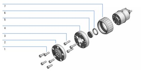
Figure 5 Valve Head Parts (example)
