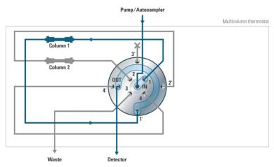
Figure 4 Hydraulic flow path schematics for 2-column selection setup with purge and valve bypass line
